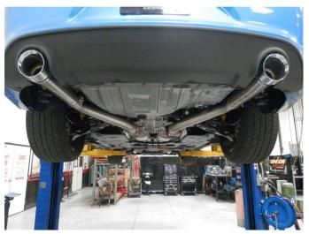
Step 5. Loosely install both Tail Pipe Assemblies using the supplied clamps. Attach the welded hangers to the rubber insulators.
