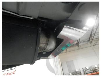
**Step 3.** Next, loosen the band clamps attaching the rear muffers to the OEM tips. Disengage all welded hangers from the rubber insulators. You may now remove the rear exhaust system. Do not discard or damage the rubber insulators as they will be used to install the new exhaust system.
