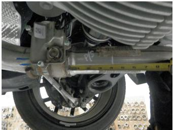
**Step 2.** For the passengers side cut 4" rearward of the outlet weld on the exhaust control valve as shown in the attached picture.
