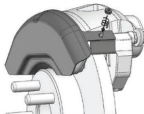
Install the supplied lock nuts onto the threaded studs to secure clip to bridge. Tighten with 3/8-inch wrench or socket to 25 in pounds. Do not overtighten nuts.
