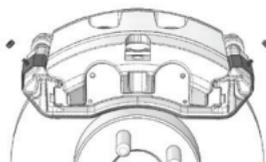
Remove lock nuts from snap clips.
