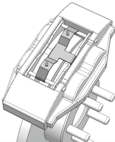
Caliper Cover should rest directly against the face of the brake caliper. The installer should verify that the bridges are set to 88° as depicted on image. Installer may adjust as needed.
