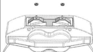
Remove lock nuts from snap clips.
