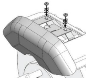
Install the supplied lock nuts onto the threaded studs to secure clip to bridge. Tighten with 3/8-inch wrench or socket to 25 in pounds. Do not overtighten nuts.
