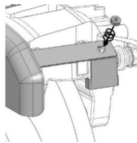
Install the supplied lock nuts
