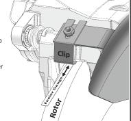
Caliper Cover should rest directly against the face of the brake caliper. The installer should verify that the bridges are set to 88°as depicted on image. Installer may adjust as needed.
