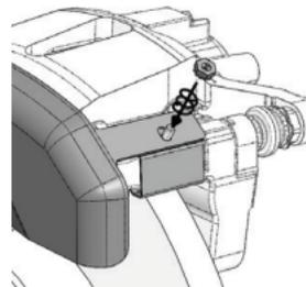
Install the supplied lock nuts
