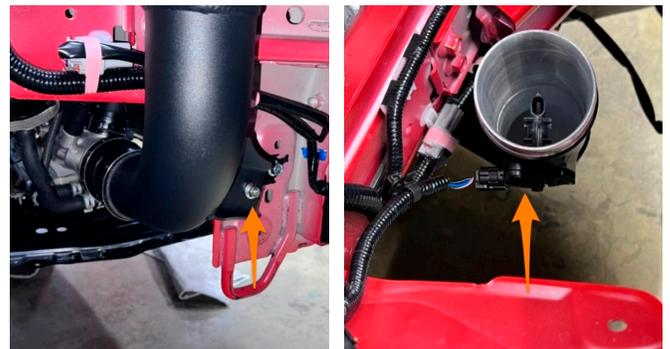
**17.** Using a 10mm socket. Install the airbox using the factory hardware and mount points.
