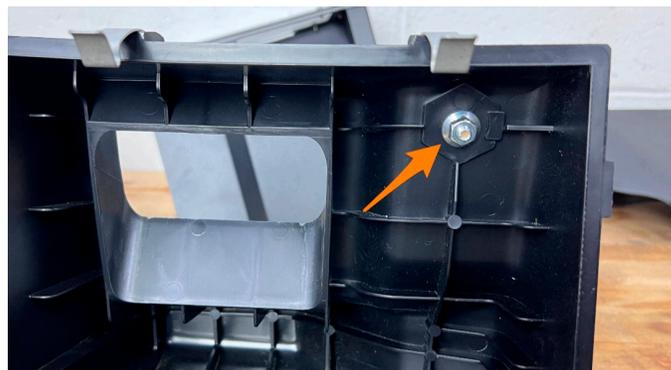
9. Remove the two rubber bushings from the airbox by first pushing the metal sleeve out.
