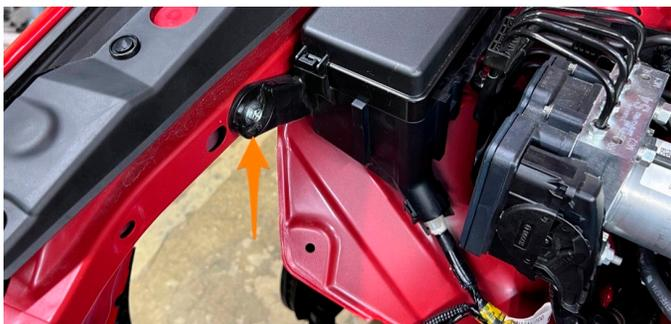
5. Using an 8mm socket, loosen the hose clamp on the intake pipe.
