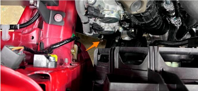
**20.** Using a 2.5mm Allen, install the airbox lid with the provided M4 hardware. Don't over-tighten. Install the factory airbox duct and pop clips.
