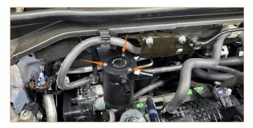
9. Install the shorter end of the supplied bent hose to the port on the catch can labeled "OUT" and secure it with one (1) of the supplied worm gear clamps. Install the other end of this hose to the port on the intake manifold and secure it with one (1) of the supplied worm gear clamps. The worm gear clamps can be tightened using a 7mm socket or a flathead screwdriver.
