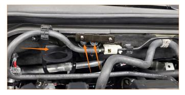
6. Place the split hose over the stock fuel hose that runs in front of the catch can bracket. Use the two (2) supplied tree clip zip ties to secure the fuel hose to the catch can bracket, as shown in the photo below.
