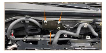
8. Using a 2.5mm Allen key, attach the Mishimoto catch can to the catch can bracket with the three (3) supplied M4 bolts.
