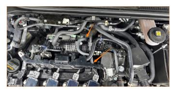
3. Using a 10mm socket, remove the two (2) nuts and one (1) bolt securing the front part of the two-piece fuel hose bracket on the firewall. Remove the front part of the bracket to gain access to the bolts securing the rear part of the bracket to the vehicle.
