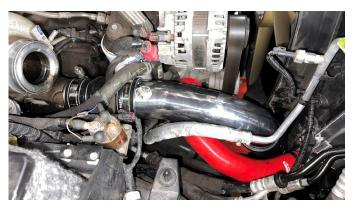
13. The cold side charge pipe and couplers are installed in the orientation shown below. Install couplers 2 and 4 onto pipe 2 in the orientation shown (label toward the pipe) and fasten with 105mm worm gear clamps. It will be installed as an assembly and adjusted once installed.
