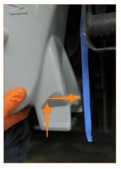
5. Working one side at a time, lift the intercooler slightly and slide the provided isolator between the intercooler and lower mount.
