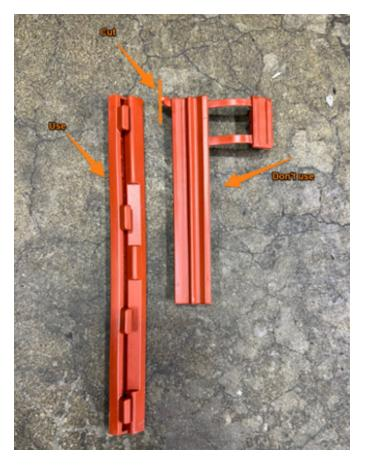
05. Install trimmed gasket onto the stock intercooler. \*NOTE: Prototype gasket shown for illustration purposes.
