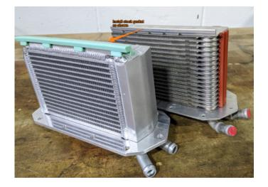
**06.** Install Mishimoto intercooler in the stock location using supplied hardware.
