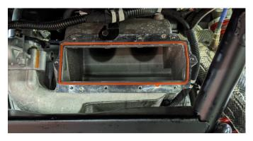
04. Remove gasket from the stock intercooler, and cut where shown. (Second image on next page)
