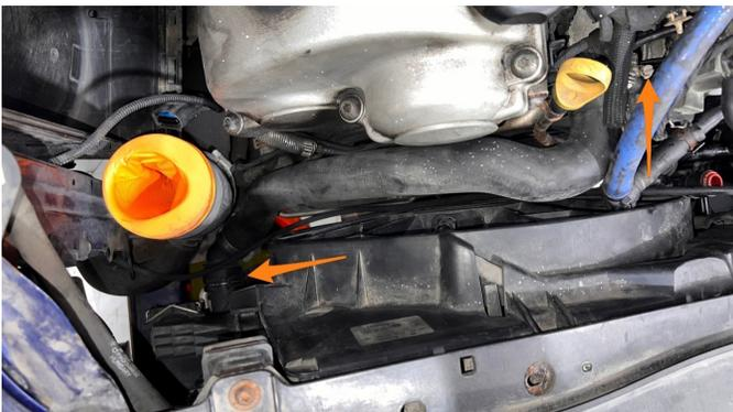
**32.** Loosen hose clamp (8mm) and remove upper hose.
