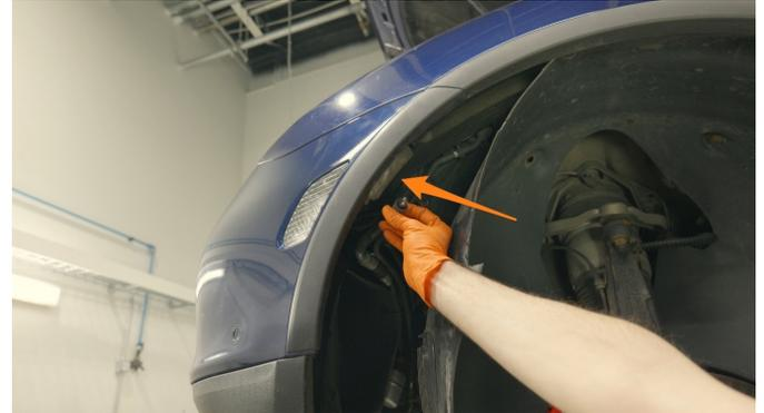
9. Remove the 2x Torx screws fastening the bumper (T30). Repeat for the other side.
