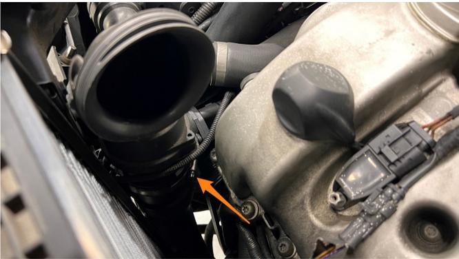
**25.** Remove upper radiator hose quick-connect fitting by releasing the clip with a pick tool then pulling the hose out.
