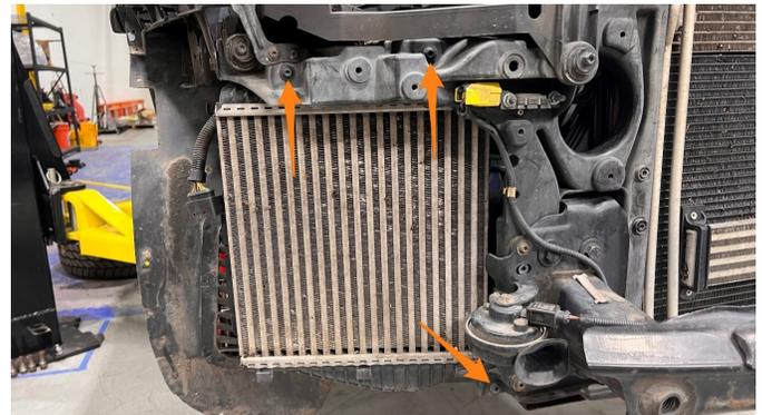
**28.** Disconnect electrical plugs for MAP sensor and throttle body, pull the 2x pins and remove Y pipe.
