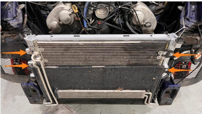
**53.** Fasten the 3 pairs of cooler lines to the radiator brackets (AC lines shown).
