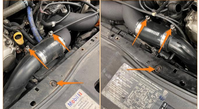
**27.** Remove the 3x Torx screws for the intercooler (T30) and pull the intercooler/pipe assembly out the side of the vehicle. Repeat for the other side.
