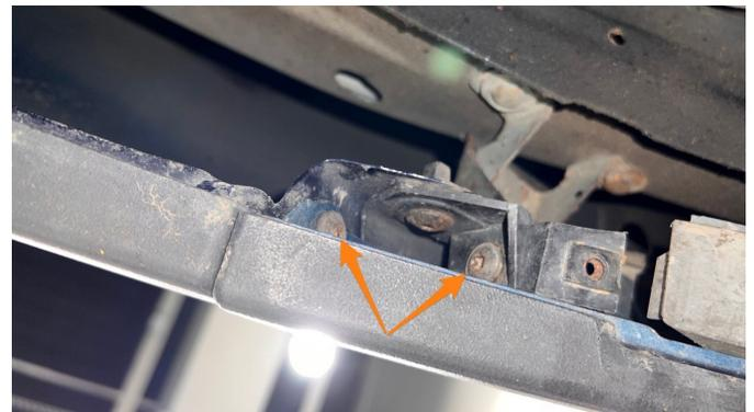
10. Remove the plastic cover by pushing down on the front-facing side.
