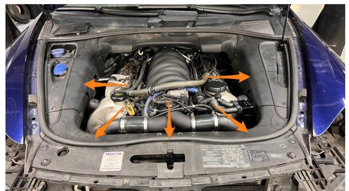
**23.** Disconnect the MAF sensor plug (1), pull the 2x pins for airbox intake pipe (2) and remove airbox lid (3) by releasing the 2x latches on the top. Remove the air filter and set aside in a clean spot. Repeat for the other side.
