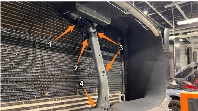
**20.** Remove the 3x Torx screws fastening the bracket (T30).
