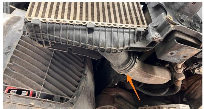
**17.** Use a pop clip tool to remove the 4x wiring harness clips from the radiator air duct.
