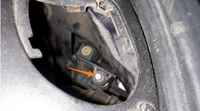
**12.** Remove the 4x upper bumper Torx bolts (T30) then remove the bumper by pulling toward the front of the vehicle. Note: the sides of the bumper near the fenders slide out toward the front. They do not pull away from the side of the vehicle like most bumpers.
