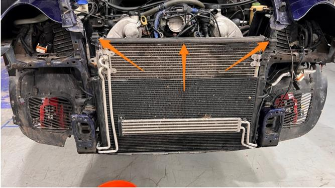
**47.** Zip-tie the top of the radiator to the frame to hold it in place then remove the lower brace that was reinstalled in step 37. Remove the clips holding the transmission cooler and AC condenser from the radiator.
