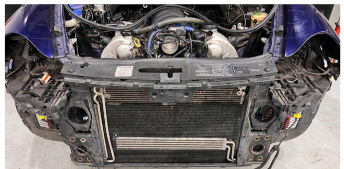
**58.** Reinstall the crash bar ensuring the tabs are properly slotted into the radiator mounts.
