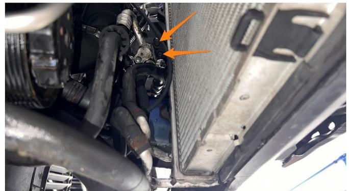
**35.** Remove the Torx screw (T30) fastening the power steering cooler lines to the radiator.
