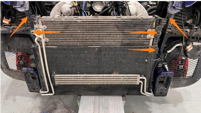
**48.** Remove the transmission cooler from the radiator and lay it down. Remove the AC condenser from the radiator and let it rest on the frame rail.
