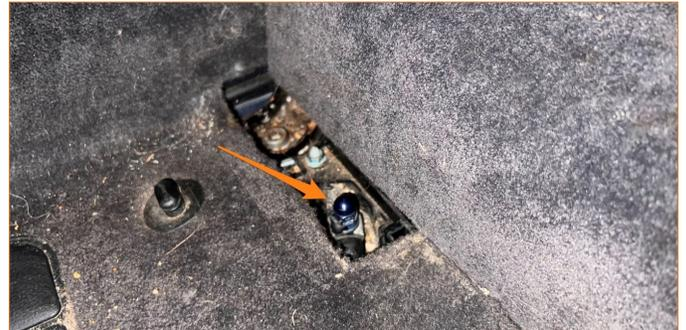
**3.** Under the vehicle, remove the 5x Torx screws (T25) then, remove the passenger side air duct. Repeat for the other side.
