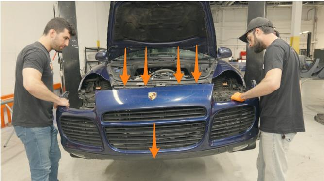
**13.** Remove the intercooler air duct by releasing the catch on the bottom then sliding it out toward the side. Repeat for the other side.
