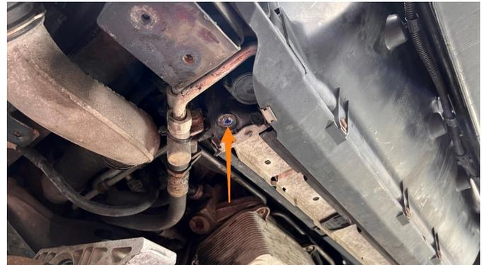
**16.** Disconnect the lower intercooler quick connect fitting by releasing the clip with a pick tool then pulling the charge pipe out. Repeat for the other side.
