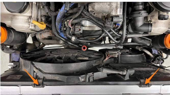
**55.** Install the provided set screws in the fan shroud clamps (2.5mm Allen) and tighten until shroud is locked in.
