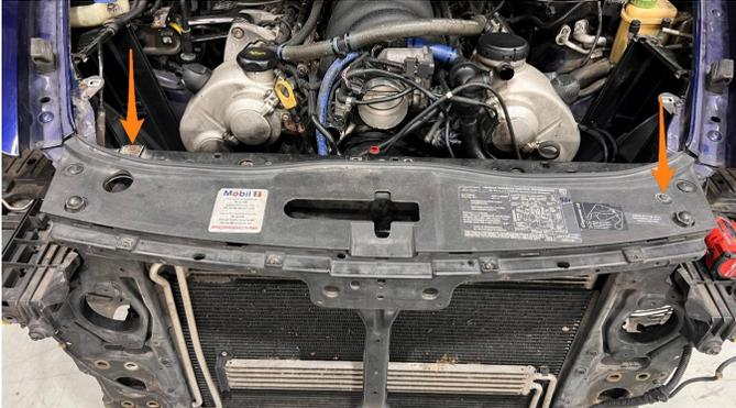
**42.** Remove the 6x Torx screws (T30) from the bumper bracket then remove the bracket. Repeat for the other side.
