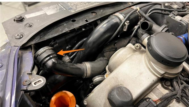
**26.** Remove the 2x Torx bolts for the charge pipes (T30), loosen the 4x hose clamps for the couplers (8mm), and remove couplers.
