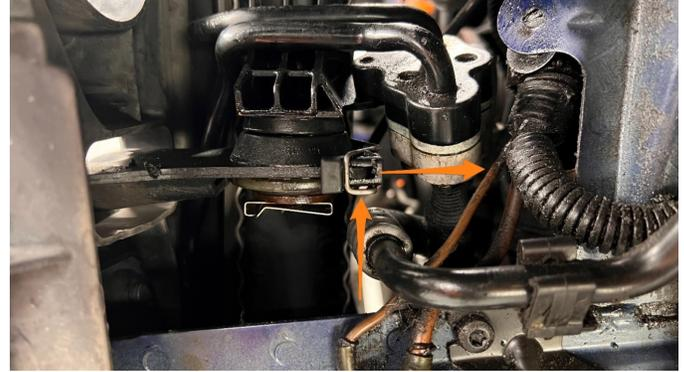
**39.** Disconnect the electrical plugs for the two horns.
