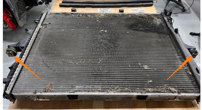
**50.** Make sure the washers are installed in the stock mounts.
