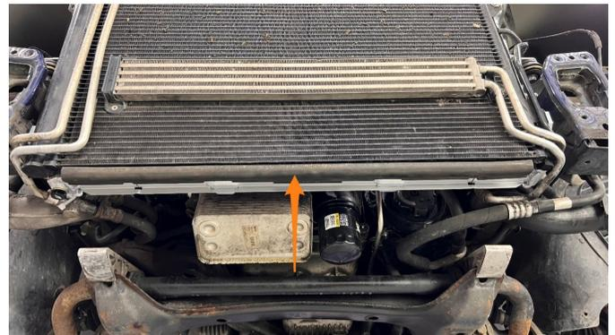
**57.** Reinstall the front core support and headlight bracket assembly by reversing removal steps.
