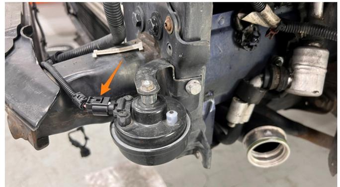
**40.** Remove the 8x bolts (16mm) and 4x Torx screws (T30) from crash bar then remove the crash bar.
