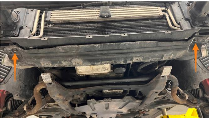
**38.** Use a pick tool to remove the metal clips from the rad mounts and then remove the black plastic caps.
