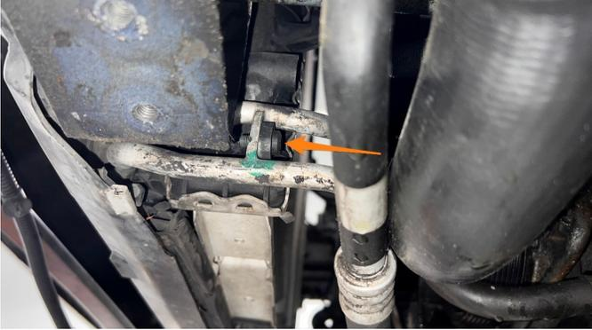
**36.** Remove the Torx screw (T30) fastening the transmission cooler lines to the radiator (missing on this vehicle).
