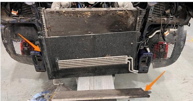
**49.** Cut the zip ties and remove the radiator from the vehicle. Remove the 2x clips for the radiator mounts then remove the mounts.
