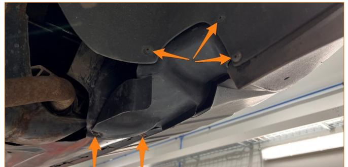
**4.** Remove the 6x bolts (10mm) then, remove the splash guard.
