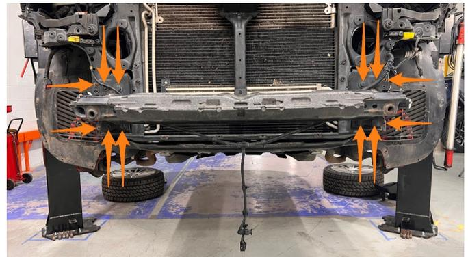
**41.** Remove the 2x upper rad mount Torx screws (T30).
