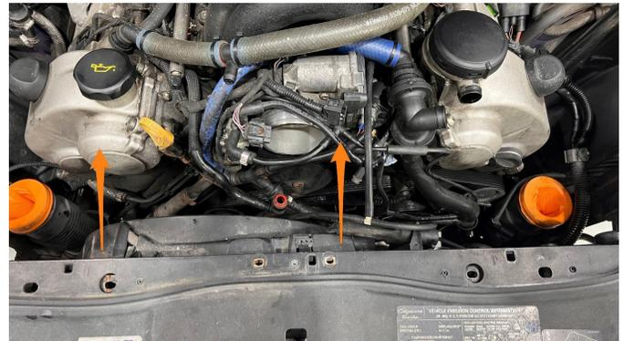
**34.** From underneath, remove the 2x Torx screws (T30) fastening the condenser lines to the radiator.
