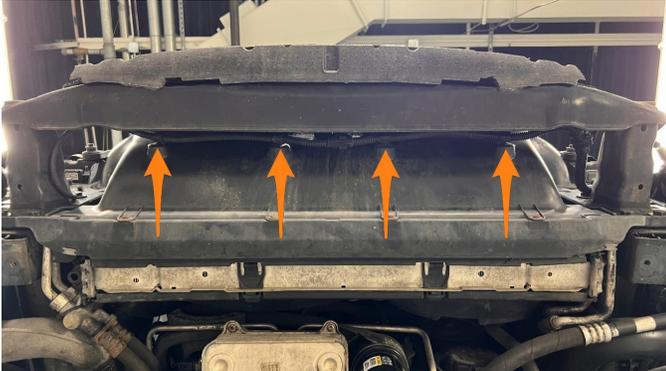
**18.** Pull the piece of foam off the intake pipe then, pull forward and rotate back and forth to release the connection from the airbox. One released, pull the intake pipe out the front. You may need to rotate them to get the pipes around other components. Repeat for the other side.
