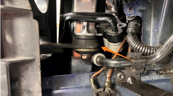
**59.** Reinstall the stock plastic retainers and metal clips onto the crash bar tabs. Make sure the radiator is pushed all the way forward and the clips are fully latched on both sides.
