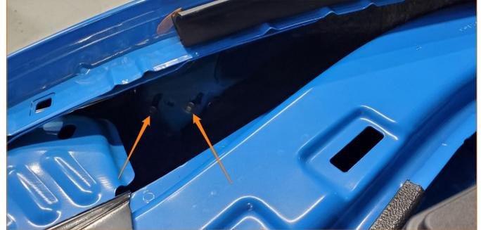
**12.** Unplug any wiring connections on the inside of the bumper (connections may vary depending on vehicle trim level and options). Then, remove the bumper from the vehicle.
