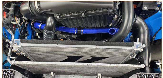
**17.** This step only applies to 2.3L vehicles. For V8 vehicles, skip to Step 18. Attach the upper mounts on the intercooler onto the hooks on the radiator. Then, push the lower intercooler mounts into the mounts on the radiator to engage the plastic clips.
