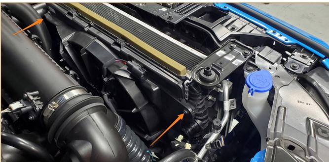
7. Using a 10mm socket, remove the two (2) bolts from each of the upper radiator mounting brackets and remove the brackets from the vehicle.
