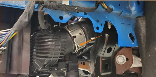
**14.** Disengage the plastic clips securing the bottom of the intercooler from the radiator and tilt the bottom of the intercooler away from the radiator. Then, lift the intercooler upwards to separate the upper intercooler mounts from the hooks on the radiator.
