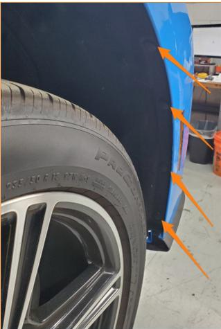
**11.** Pull back the wheel liner to access the tree clip in the upper corner of the bumper and, using a flathead screwdriver, remove the tree clip from both sides of the vehicle. Using a 10mm socket, remove the two (2) bolts inside the fender that secure the bumper to the vehicle on both sides of the vehicle.
