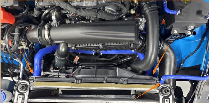
5. Disengage the red locking tab on the fan plug and disengage the plug. Then, remove the tree clips from the fan shroud to separate the wiring harness from the shroud.
