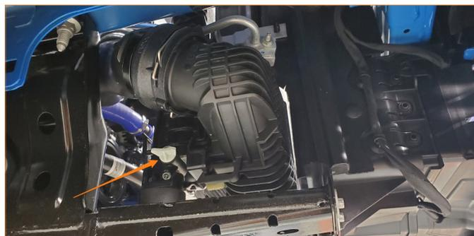
3. Using pop clip pliers or a flathead screwdriver, remove the eight (8) pop clips from the radiator cover and remove the cover from the vehicle.
