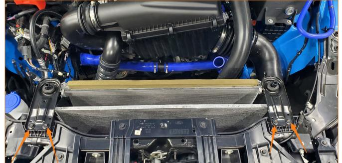
8. Using a 10mm wrench, remove the one (1) bolt securing the A/C condenser to the radiator. Then, disengage the plastic clip securing the tab on the other side of the A/C condenser and lift the condenser straight up to separate the tabs on the condenser from the hooks on the radiator. Depending on the vehicle trim level and options, additional coolers may be present. If so, separate them from the radiator the same way as the A/C condenser.
