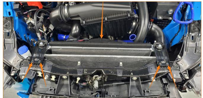
20. Using a 10mm socket, secure the fan shroud to the Mishimoto radiator using two (2) of the supplied M6 washers and bolts. Then, reconnect the fan plug, engage the locking tab, and insert the two tree clips into the holes on the fan shroud to secure the wiring harness.
