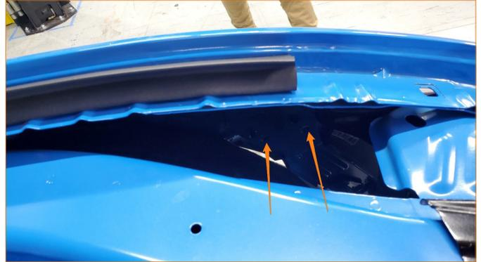
**24.** Using a 10mm socket, reinstall the six (6) bolts that were removed from the bumper in Step 9.
