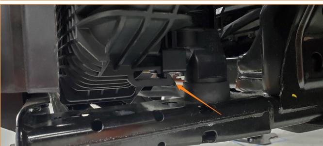
**15.** Remove the radiator from the vehicle by lifting it straight up. If the rubber grommets remained attached to the lower mounting pegs on the radiator, remove them and reinstall them into the vehicle's frame.
