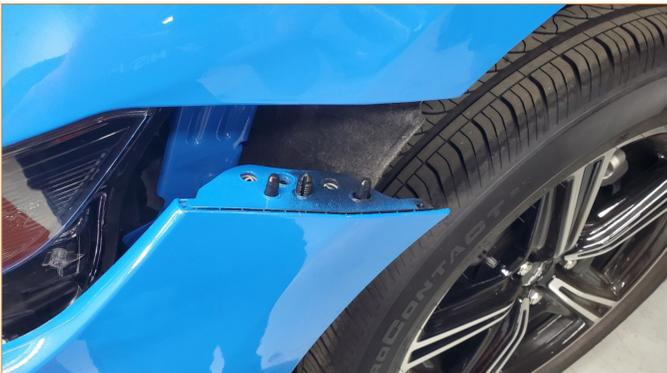
**23.** Using a 10mm socket, reinstall the four (4) bolts that were removed in Step 11 – two (2) on each side of the vehicle.
