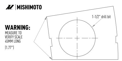
Place drilling template on inside (unpainted side) of tow hook cover.
