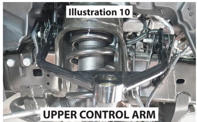
30. Attach the upper control arm to the knuckle. [21mm] (46)
