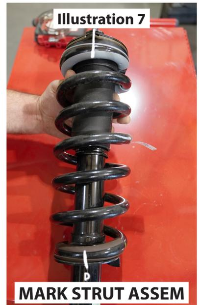
17. [Illustration 7] Mark the orientation of the strut top plate and the strut body.
