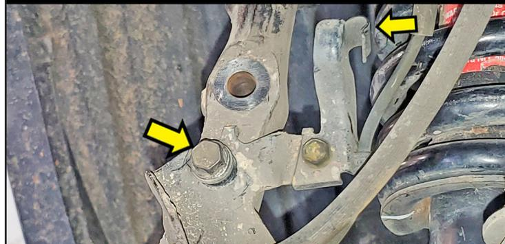
at the upper mount tab. Carefully bend the tab open with a flat screw driver taking care not to damage the abs line.
