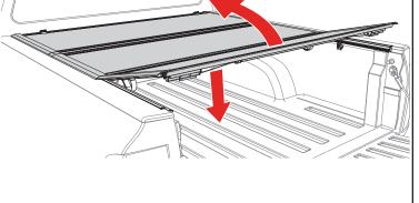
FOLDED UP POSITION: To drive with the cover (C) in the folded up position, use the straps and buckles provided with the cover. Attach the buckle at the bulkhead, then pull the strap to take up the slack and secure the cover.
