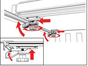
Unfold the cover (C) towards the tailgate. Then confirm each panel is centered side to side and front to back on the truck bed. If adjustments are needed, loosen the cover retainer clamps (F) and shift the cover (C) until positioned correctly. Retighten the cover retainer clamps once the desired fitment is reached. If adjustments to the slam latch are needed, see the directions on the next page. Power Tailgates: If your truck has a
