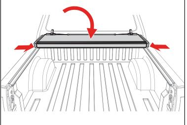
**9** Confirm the retainer clamps (F) are positioned around the side rails (A & B) correctly as shown below. Tighten the retainer clamps by turning them clockwise until the lock washer is secure.
