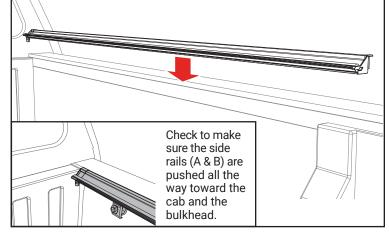
**6** For the best (C) fit, the side rails (A & B) should be level with the truck bed cap and not angled up or down. Insert the backside of the clamp as high as possible and tighten clamp. Depending on model the notch will vary. Tighten all clamps to 10 ft/lbs of torque with a 1/2" wrench or socket. **Caution: Do NOT overtighten!**
