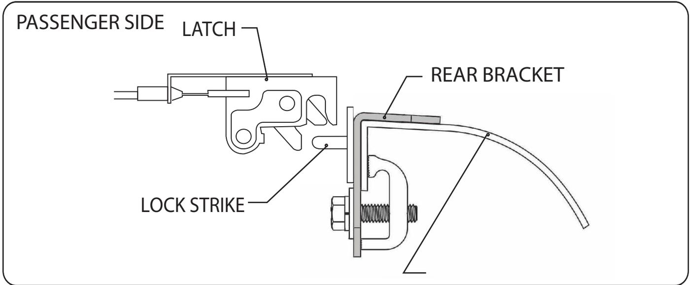
It may be necessary to adjust the latch side to side, to do so loosen the two latch mounting bolts, adjust latch and tighten.
