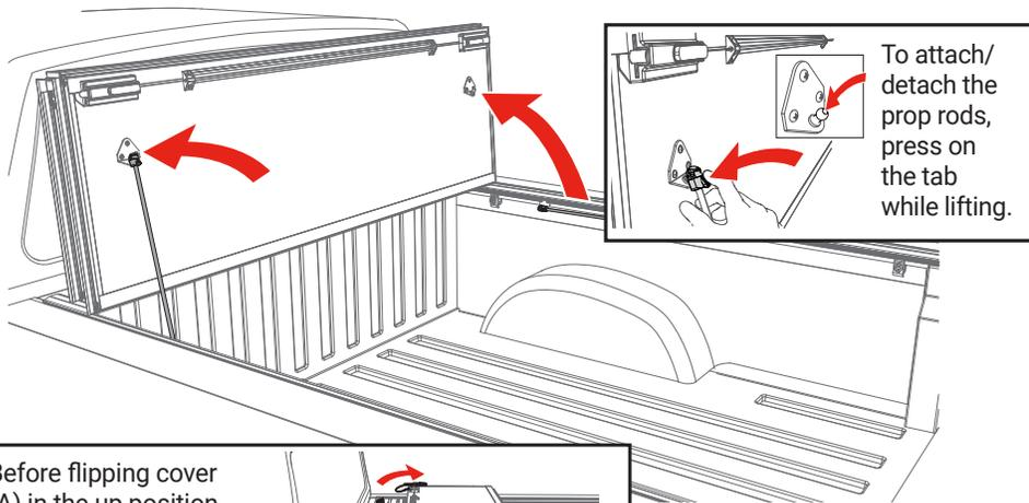
Before flipping cover (A) in the up position make sure to stow the straps using the clips on the underside of the folded cover.
