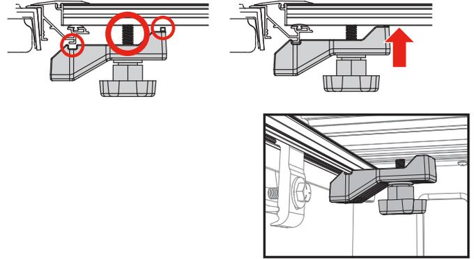
**10** Unfold the hard folding cover (A) towards the tailgate. Then confirm each panel is centered side to side and front to back on the truck bed. If adjustments are needed, loosen the cover retainer clamps (H) and shift the hard folding cover (A) until positioned correctly. Re-tighten the cover retainer clamps once the desired fitment is reached. *If adjustments to the slam latch are needed, see the directions on the next page.*
