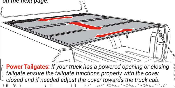
**Power Tailgates:** If your truck has a powered opening or closing tailgate ensure the tailgate functions properly with the cover closed and if needed adjust the cover towards the truck cab.
