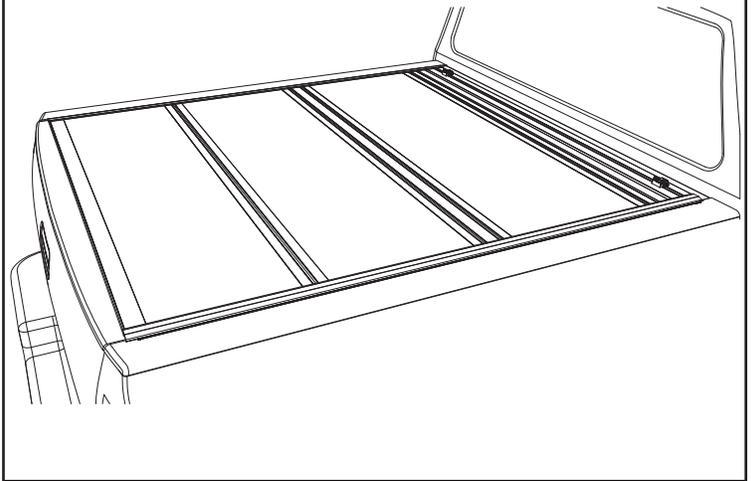
**OPENING COVER:** Lower the tailgate and pull the cable on either side. While pulling on the cable lift the panel up and towards the cab.
