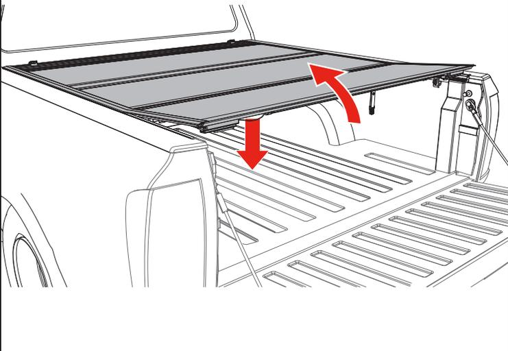
**FOLDED UP POSITION:** To drive with the cover (A) in the folded up position, use the straps and buckles provided with the cover. Attach the buckle at the bulkhead, then pull the strap to take up the slack and secure the cover.
