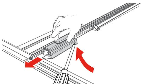
If adjustment is needed, use a straight screwdriver to partially pry open the tab on the latch housing. At the same time slide the housing away from the latch assembly.
