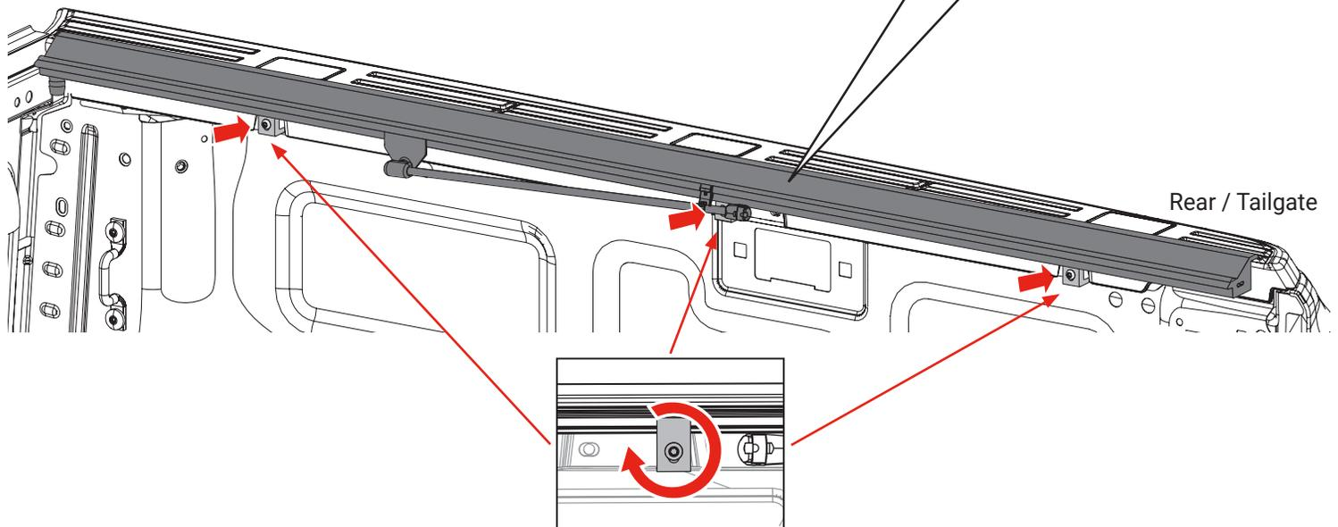
**4** For the best (B) fit, the side rails (B & C) should be level with the truck bed cap and not angled up or down.
