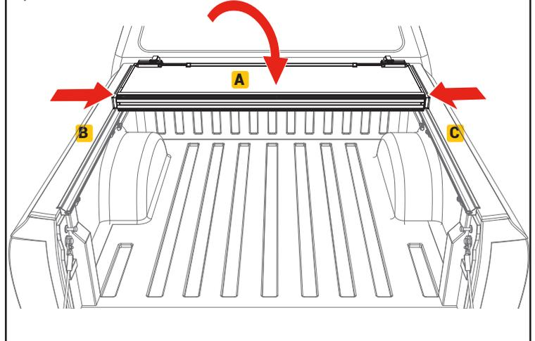
**9** Confirm the retainer clamps (H) are positioned around the side rails (B & C) correctly as shown below. Tighten the retainer clamps by turning them clockwise until the lock washer is secure.
