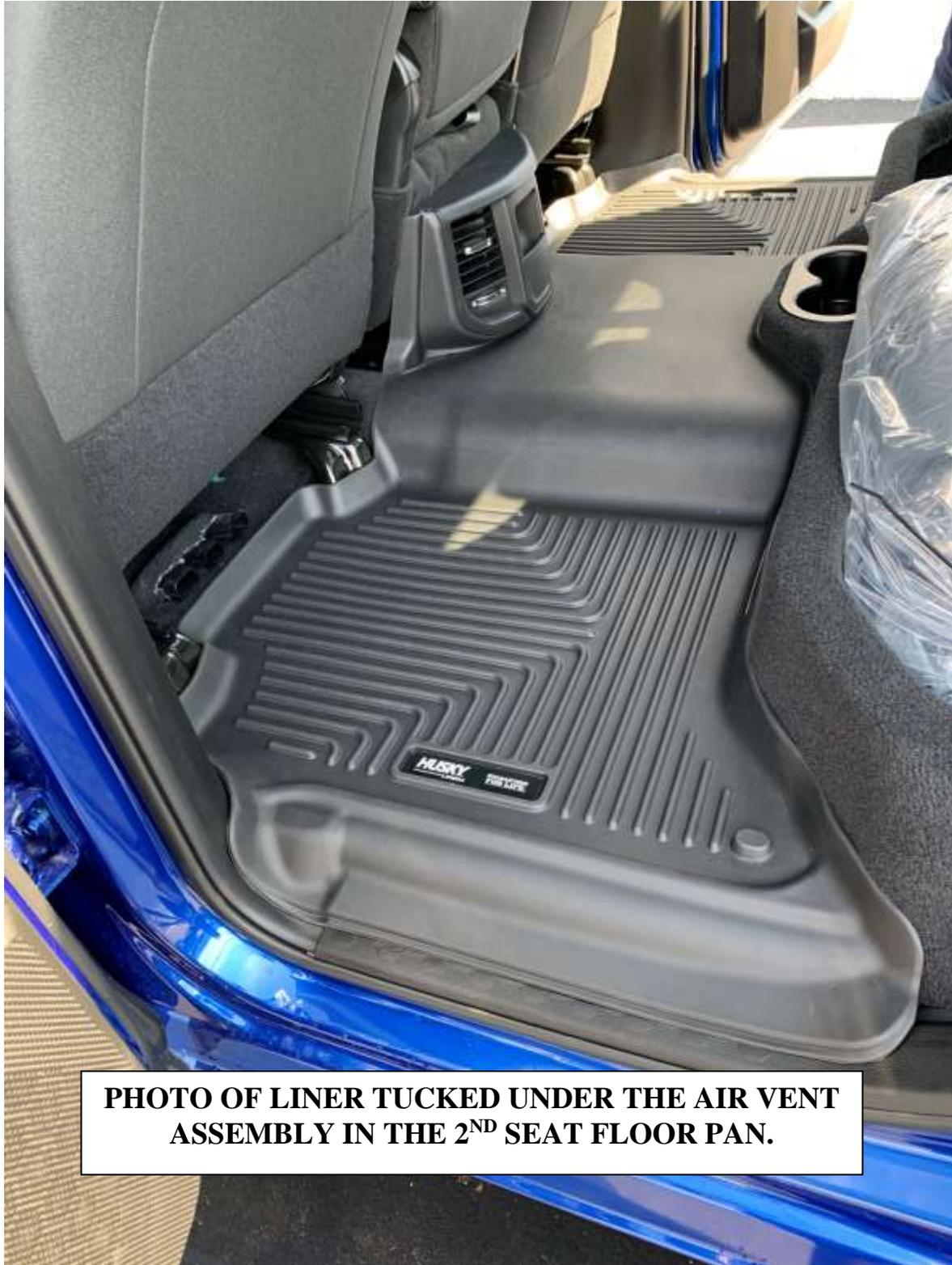
**PHOTO OF LINER TUCKED UNDER THE AIR VENT ASSEMBLY IN THE 2<sup>ND</sup> SEAT FLOOR PAN.**
