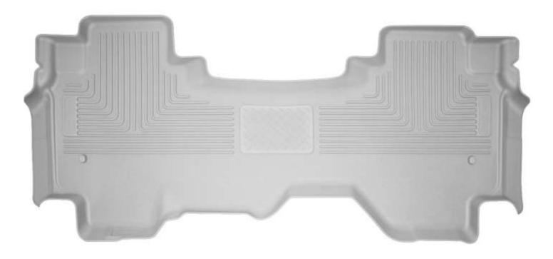
PRIOR TO INSTALLING YOUR 2<sup>nd</sup> SEAT LINER, SLIDE BOTH FRONT ROW SEATS COMPLETELY FORWARD. WITH THIS DONE, INSTALL THE LINER, POSITIONING IT AS SHOWN ABOVE. ONCE THE LINER IS IN PLACE, REPOSITION THE FRONT SEATS AS DESIRED. THE LINER TUCKS UNDER THE AIR DUCTS THAT ARE LOCATED UNDER THE BACK OF THE FRONT SEATS (SEE PHOTO ON BACK OF PAGE).
