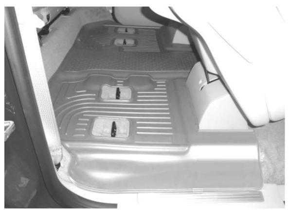
PART #1928 SHOWN INSTALLED—NOTE SEAT ATTACHES TO FLOOR THROUGH LINER
