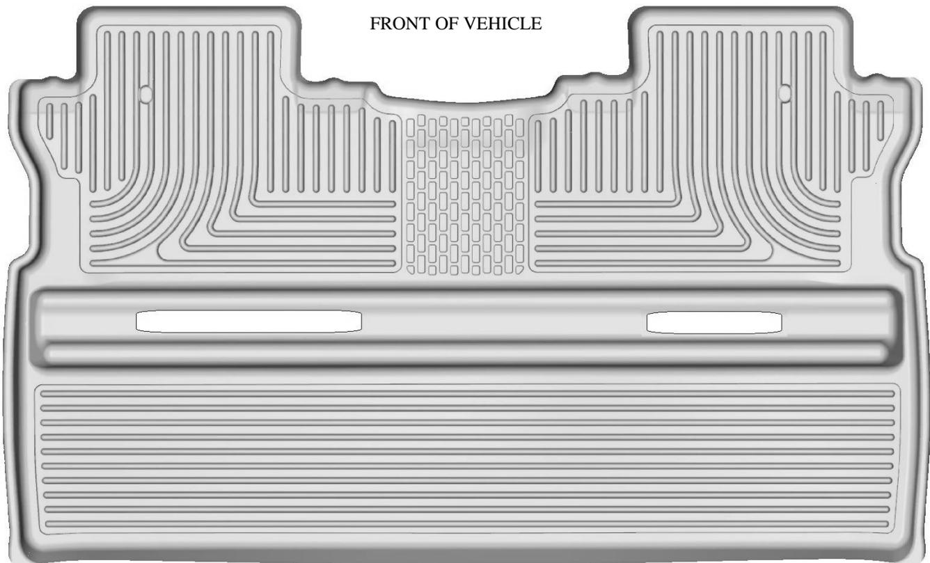
TO EASE INSTALLATION OF YOUR NEW 2<sup>ND</sup> SEAT RIDGELINE LINER, FIRST FOLD THE 2<sup>ND</sup> ROW SEATS UP. WITH THIS DONE, INSTALL YOUR LINER, POSITIONING IT AS SHOWN ABOVE. ONCE THE LINER IS INSTALLED, FOLD THE 2<sup>ND</sup> ROW SEATS BACK DOWN. NOTE THE SEAT SUPPORT BARS WILL PASS THROUGH THE TWO TRIMMED SLOTS IN LINER AS THEY LOCK INTO PLACE.
