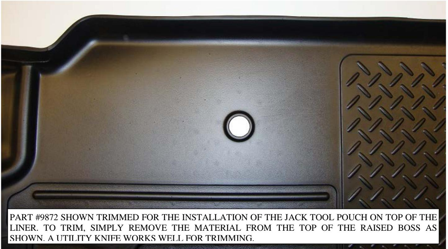
PART #9872 SHOWN TRIMMED FOR THE INSTALLATION OF THE JACK TOOL POUCH ON TOP OF THE LINER. TO TRIM, SIMPLY REMOVE THE MATERIAL FROM THE TOP OF THE RAISED BOSS AS SHOWN. A UTILITY KNIFE WORKS WELL FOR TRIMMING.
