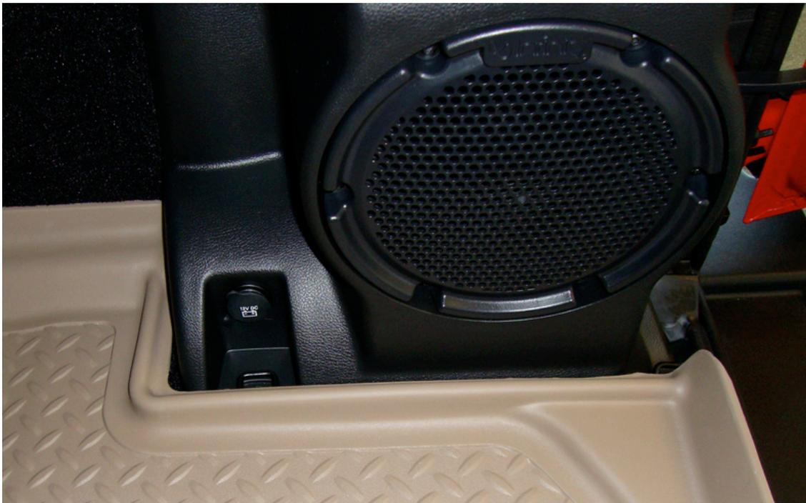
LINER SHOWN TRIMMED TO ACCESS THE CARGO TIE-DOWN HOOK LOCATIONS AND ALSO TO ALLOW INSTALLATION OF 2<sup>ND</sup> ROW SEAT ON TOP OF LINER.
