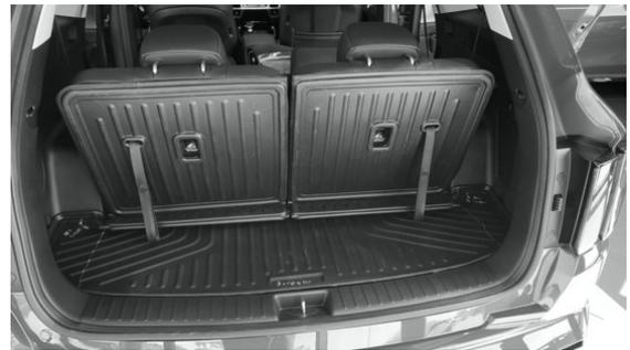
6. The liner at this point is fully installed and is ready to use. If the liner needs to be removed, grab the rectangular Velcro patches and hold them firmly in place as you pull the liner from the seat. This Velcro piece is intended to stay attached to the seat back and cargo floor to reduce wear from the liner being installed and reinstalled for cleaning.
