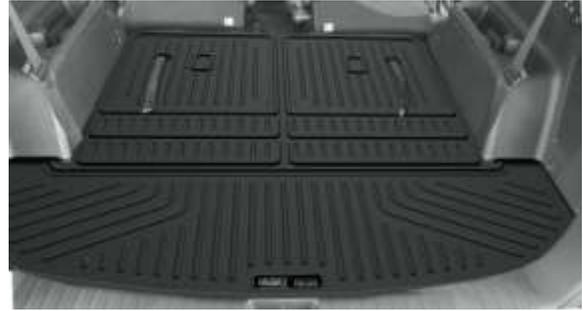
5. The first time the rear seat backs are moved to the upright position, move the seats slowly taking care to ensure the accordion section of the liner folds outward as shown. This may need to be assisted from the backside.
