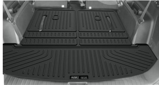
5. The first time the rear seat backs are moved to the upright position, move the seats slowly taking care to insure the accordion section of the liner folds outward as shown. This may need to be assisted from the backside.
