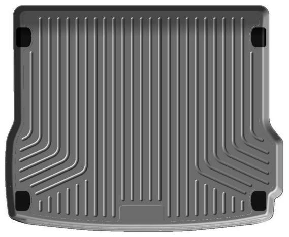
YOU CAN ACCESS THE FACTORY CARGO TIE-DOWN LOCATIONS WITH YOUR LINER IN PLACE. TO DO SO, SIMPLY TRIM AWAY THE LOWERED AREAS IN THE LINER LOCATED ABOVE THE CARGO HOOKS YOU WISH TO EXPOSE. THE FOUR HOOK LOCATIONS ARE SHOWN ABOVE DARKENED. A UTILITY KNIFE WORKS WELL FOR TRIMMING.
