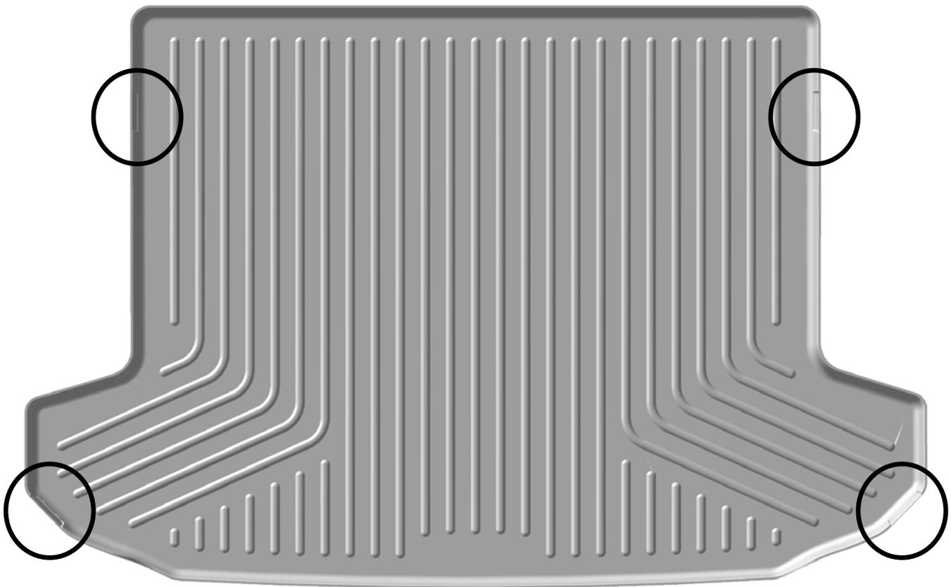
YOUR SPORTAGE HAS FOUR (4) CARGO TIE DOWN HOOKS LOCATED AROUND THE PERIMTER OF THE CARGO AREA. TO ACCESS TO THE FACTORY TIE-DOWN HOOK LOCATIONS (SHOWN CIRCLED ABOVE) WITH THE LINER IN PLACE. SIMPLY REMOVE/TRIM THE MATERIAL FROM THE PORTION OF THE LINER OVERLAPPING THE HOOKS. THESE AREAS ARE RECESSED ON THE LINER TO GUIDE TRIMMING. A UTILITY KNIFE WORKS WELL FOR TRIMMING.
