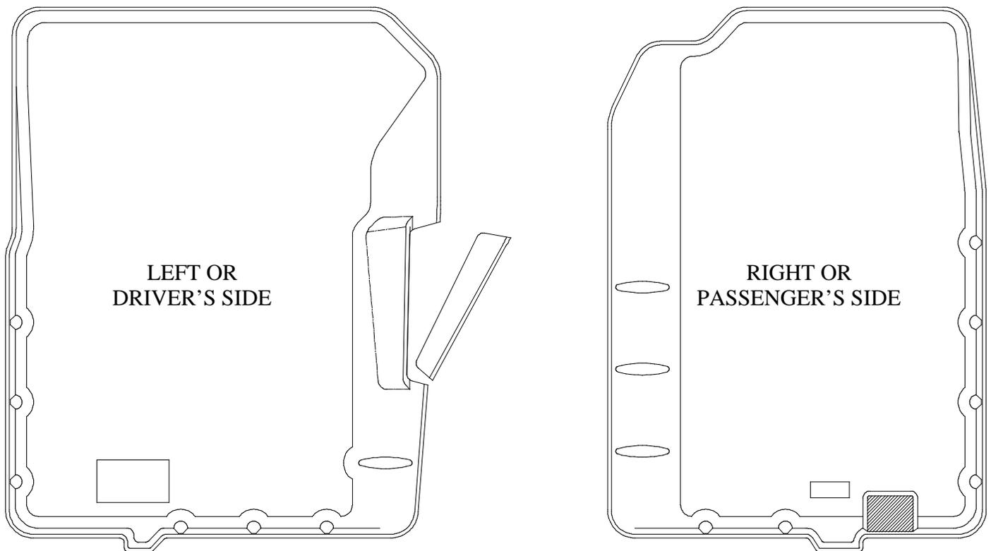
IF YOUR VEHICLE IS EQUIPPED WITH A MANUAL TRANSFER CASE SHIFTER, YOU WILL NEED TO TRIM YOUR DRIVER'S SIDE LINER AS SHOWN ABOVE. TRIM AWAY THE RECESSED PORTION ON THE LINER WALL. SOME CREW CAB MODELS MAY REQUIRE THE RAISED AREA SHOWN DARKENED ON THE PASSENGER'S SIDE LINER TO BE TRIMMED AWAY TO ALLOW PROPER FIT. A UTILITY KNIFE OR HEAVY SCISSORS WORKS WELL FOR TRIMMING.
