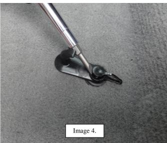
2) WITH THE FACTORY CLIPS REMOVED, UNSCREW THE TWO HALVES OF THE HUSKY® RETAINING CLIP AND INSERT THE BOTTOM HALF INTO THE EXISTING FACTORY GROMMETS LOCATION AS SHOWN BELOW IN IMAGE 4 AND IMAGE 5. THE BOTTOM PORTION WILL "SNAP" SECURELY INTO THE FACTORY GROMMET LOCATION. RETAIN THE TOP HALF OF THE CLIP FOR LATER INSTALLATION.
