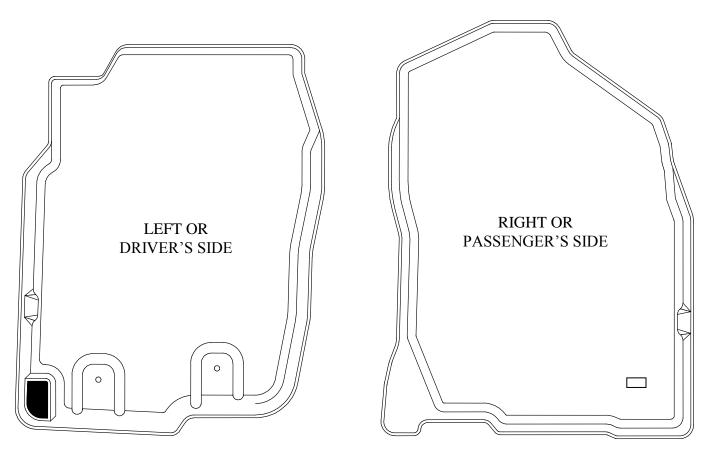
IF YOUR VEHICLE IS EQUIPPED WITH A FLOOR MOUNTED FUEL DOOR RELEASE LEVER, YOUR LINER CAN EASILY BE TRIMMED TO ALLOW ACCESS TO THE LEVER. JUST TRIM AWAY THE MATERIAL FROM THE AREA SHOWN ABOVE DARKENED. THE AREA IS SLIGHTLY RECESSED TO PROVIDE A TRIMMING GUIDE. TO TRIM, USE A UTILITY KNIFE OR SIMILAR ITEM.
