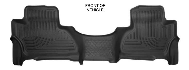
TO EASE INSTALLATION OF YOUR SECOND SEAT LINER, MOVE THE FRONT SEATS TO THEIR MOST FORWARD POSITIONS. WITH THIS DONE, INSERT LINER IN VEHICLE ANGLING THEM SO THAT THE FRONT EDGE OF THE LINER IS SEATED INTO PLACE FIRST, THEN LOWER THE REAR OF THE LINER. ONCE THE LINER IS INSTALLED, REPOSITION THE FRONT SEATS AS DESIRED.
