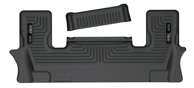
TO EASE INSTALLATION OF YOUR NEW LINERS, MOVE BOTH SECOND ROW SEATS TO THEIR MOST FORWARD POSITION. WITH THIS DONE, INSTALL THE LINERS AS SHOWN ABOVE. ONCE YOU HAVE INSTALLED YOUR LINERS, REPOSITION THE SEATS AS DESIRED.
