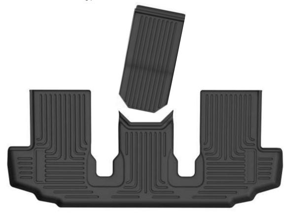
TO EASE INSTALLATION OF YOUR NEW THIRD SEAT LINER, FLIP AND SLIDE FORWARD THE SECOND ROW SEATS TO ALLOW EASY ACCESS TO THE THIRD ROW FLOOR. POSITION THE LINER AS SHOWN ABOVE. ONCE THE LINER IS IN PLACE, MOVE THE SECOND SEATS BACK TO THE DESIRED POSITIONS.
