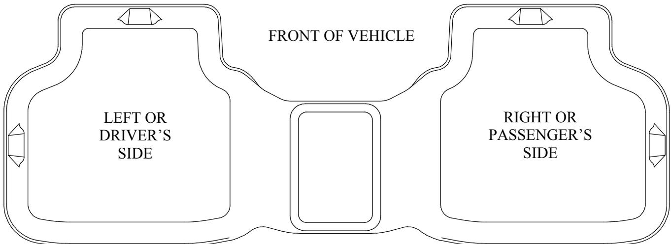
TO EASE INSTALLATION OF YOUR DODGE JOURNEY SECOND SEAT LINER, MOVE BOTH FRONT SEATS TO THEIR MOST FORWARD POSITION BEFORE INSTALLING LINER. ONCE LINER IS IN PLACE, REPOSITION THE FRONT SEATS AS DESIRED.
