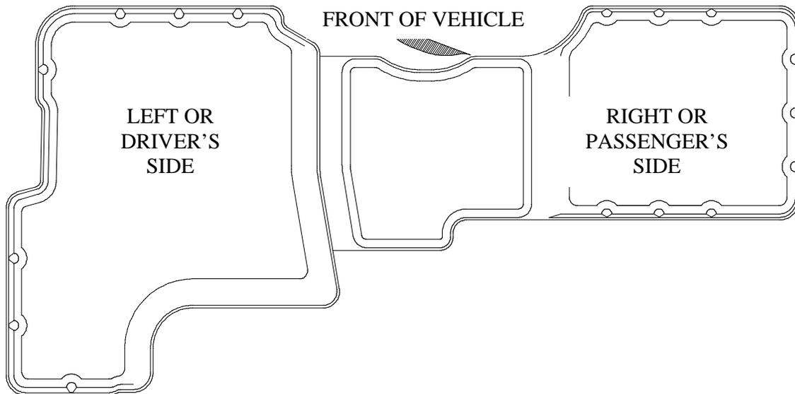
ON VEHICLES EQUIPPED WITH A CENTER CONSOLE IT WILL BE NECESSARY TO TRIM YOUR LINER AS SHOWN ABOVE. USE THE EDGE OF THE RAISED BAND AS A TRIMMING GUIDE. A UTILITY KNIFE WORKS WELL.
