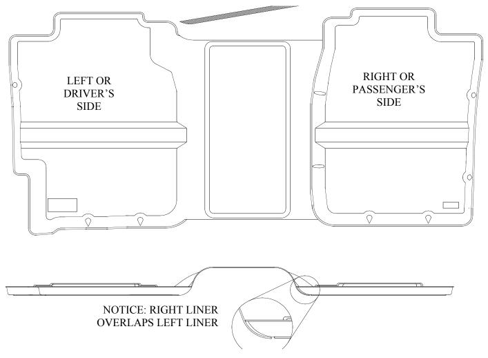
SOME SILVERADO/SIERRA OWNERS WILL NEED TO TRIM THEIR DRIVER'S SIDE LINER AS SHOWN ABOVE (TOP) TO ALLOW FOR AN OPTIONAL LONGER CENTER CONSOLE (BETWEEN THE TWO FRONT BUCKET SEATS). TRIM AWAY THE LOWERED AREA (WHERE THE LINER MEETS THE CONSOLE) USING THE OFFSET STEP IN THE LINER AS A GUIDE. A UTILITY KNIFE OR HEAVY SHEARS WORK WELL FOR TRIMMING
