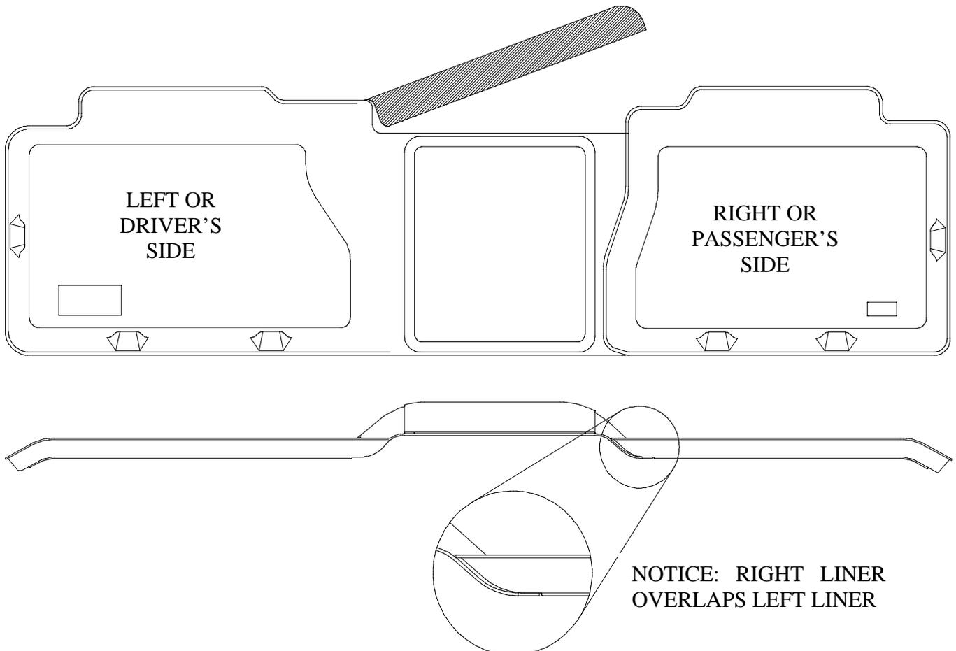
YUKON DENALI OWNERS WILL NEED TO TRIM THEIR LINER TO ACCOMMODATE THE FACTORY EQUIPPED CONSOLE. TRIM AWAY THE MATERIAL ON THE LINER THAT IS LOWERED AS DEMONSTRATED ABOVE AND AS SHOWN ON THE PHOTOS ON THE REVERSE SIDE.
