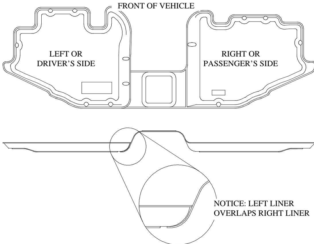
SOME 2000 MODEL YEAR WRANGLER'S HAVE A FULL CENTER CONSOLE THAT WILL INTERFERE WITH THE PORTION OF THE LINER DESIGNED TO COVER THE VEHICLE'S "HUMP" AREA. THIS PORTION CAN BE EASILY TRIMMED AWAY USING A UTILITY KNIFE OR HEAVY SHEARS. TRIM ALONG THE STEP MOLDED INTO THE PASSENGER SIDE "HUMP" WALL LEAVING THE TOP OF THE STEP AS A "LIP." SEE DIAGRAM AT RIGHT. PHOTOS OF A TRIMMED PART ARE ON SHOWN ON THE BACK OF THIS INSTRUCTION SHEET.
