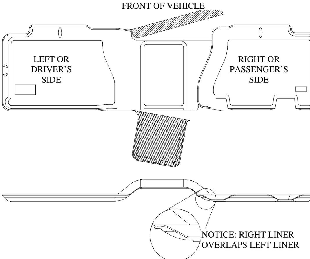
YUKON DENALI XL OWNERS WILL NEED TO TRIM THEIR DRIVER'S SIDE LINER AS SHOWN ABOVE TOP TO ALLOW FOR THE LARGER CENTER CONSOLE (SEE PHOTOS ON BACK). TRIM AWAY THE LOWERED AREA ON THE LINER. A UTILITY KNIFE OR HEAVY SHEARS WORK WELL FOR TRIMMING. ON VEHICLES EQUIPPED WITH A REAR BENCH SEAT, A PORTION OF THE SECOND SEAT LINER (SHOWN ABOVE HATCHED) CAN BE TRIMMED OFF TO ALLOW EASIER INSTALLATION AND REMOVAL. TRIM ALONG THE EDGE OF THE BAND BISECTING THE CENTER PORTION
