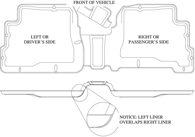
TACOMA'S EQUIPPED WITH A CENTER CONSOLE WILL NEED TO HAVE THEIR HUSKY LINERS TRIMMED TO ALLOW PROPER FIT. TRIM LINER FOLLOWING THE SCRIBED LINES ON THE PASSENGER SIDE LINER'S HUMP PORTION, PASSING APPROXIMATELY \_" ABOVE THE RAISED BAND BISECTING THE TREADED AREA ON THE HUMP (SEE ABOVE). A UTILITY KNIFE OR HEAVY SHEARS WORK WELL FOR TRIMMING. A PHOTO ON THE BACK SHOWS A TRIMMED PART.
