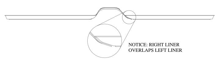
TUNDRA OWNERS WITH THE POWER SEAT OPTION WILL NEED TO TRIM THEIR DRIVER'S SIDE LINER TO ALLOW CLEARANCE OF THE POWER SEAT TRACK (SEE ABOVE). REMOVE THE MATERIAL FROM THE TWO RAISED AREAS. A UTILITY KNIFE OR SCISSORS WORK WELL.
