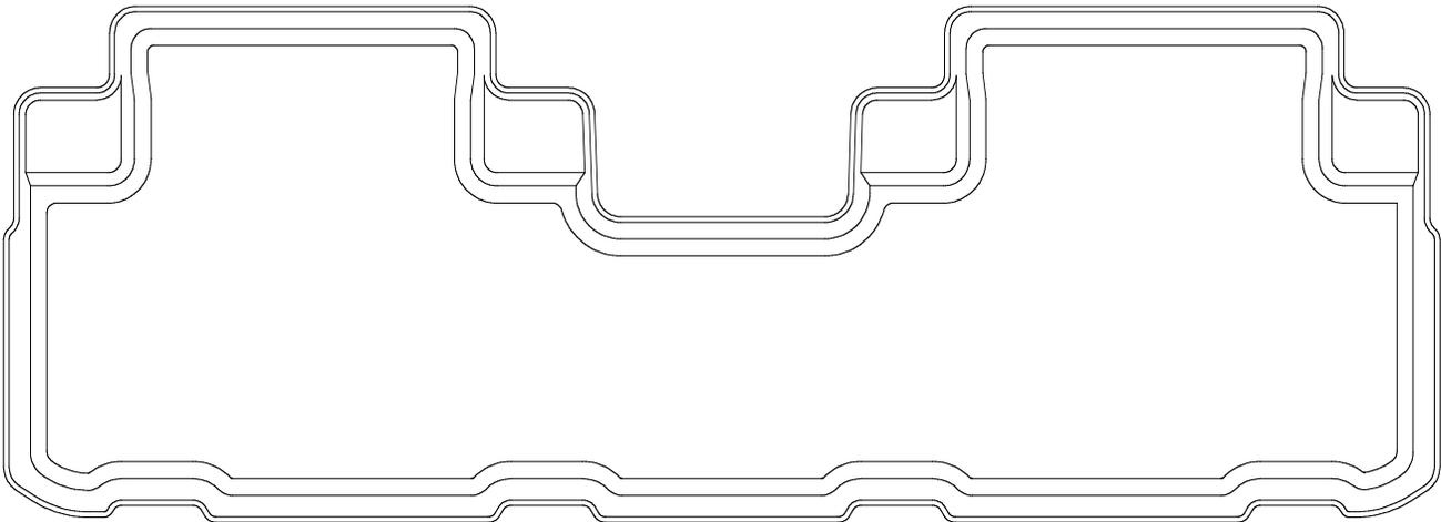
TO EASE INSTALLATION OF YOUR NEW HUSKY SECOND SEAT LINER, ADJUST BOTH FRONT SEATS TO THEIR MOST FORWARD POSITION. ONCE THIS IS COMPLETED, INSTALL LINER AS DEPICTED ABOVE THEN REPOSITION FRONT SEATS AS DESIRED.
