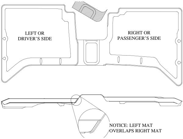
DUE TO DIFFERENCES IN AVAILABLE CONSOLE CONFIGURATIONS, 2000/2001 XTERRA OWNERS MAY NEED TO TRIM THEIR LINER AS SHOWN ABOVE. THE TRIMMING NECESSARY IS EASILY DONE BY FOLLOWING THE SCRIBED LINE MOLDED INTO THE PART. A UTILITY KNIFE OR SCISSORS WORK WELL FOR TRIMMING. PHOTOS OF TRIMMED AND UNTRIMMED PARTS ARE INCLUDED ON BACK.
