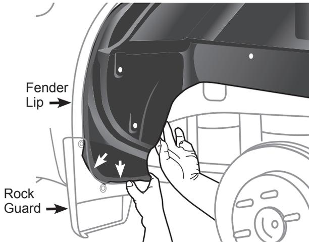
**6** Tuck the lower tail part of the wheel well liner behind the metal lip of truck's fender. Also tuck it behind the factory rock guard.
