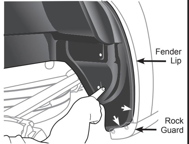
**7** Tuck the upper part of the wheel well liner behind the rest of the metal lip of the truck's fender.
