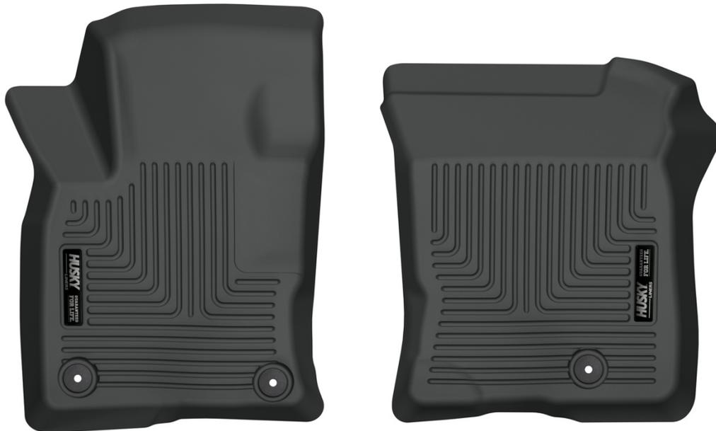
TO EASE INSTALLATION OF YOUR NEW FRONT LINERS, MOVE BOTH FRONT ROW SEATS TO THEIR MOST REARWARD POSITION. WITH THIS DONE, INSTALL THE LINERS AS SHOWN ABOVE. THE DRIVERS SIDE LINER HAS TWO HOLES WHICH SNAP OVER THE FACTORY MAT RETAINERS. ONCE YOU HAVE INSTALLED YOUR LINERS, REPOSITION THE SEATS AS DESIRED.
