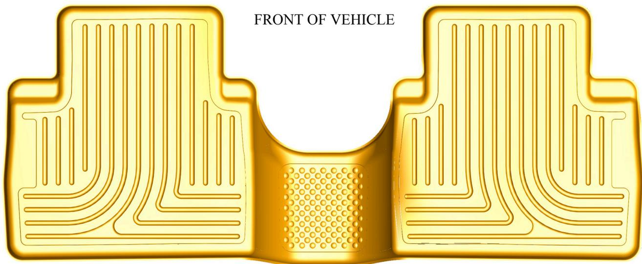
TO EASE INSTALLATION OF YOUR ACCORD SECOND SEAT LINER, MOVE THE FRONT SEATS TO THEIR MOST FORWARD POSITIONS. WITH THIS DONE, INSERT LINER IN VEHICLE ANGLING IT SO THAT THE BACK EDGE OF THE LINER IS SEATED INTO PLACE FIRST, THEN LOWER FRONT PORTION. ONCE LINER IS INSTALLED, REPOSITION THE FRONT SEATS AS DESIRED.
