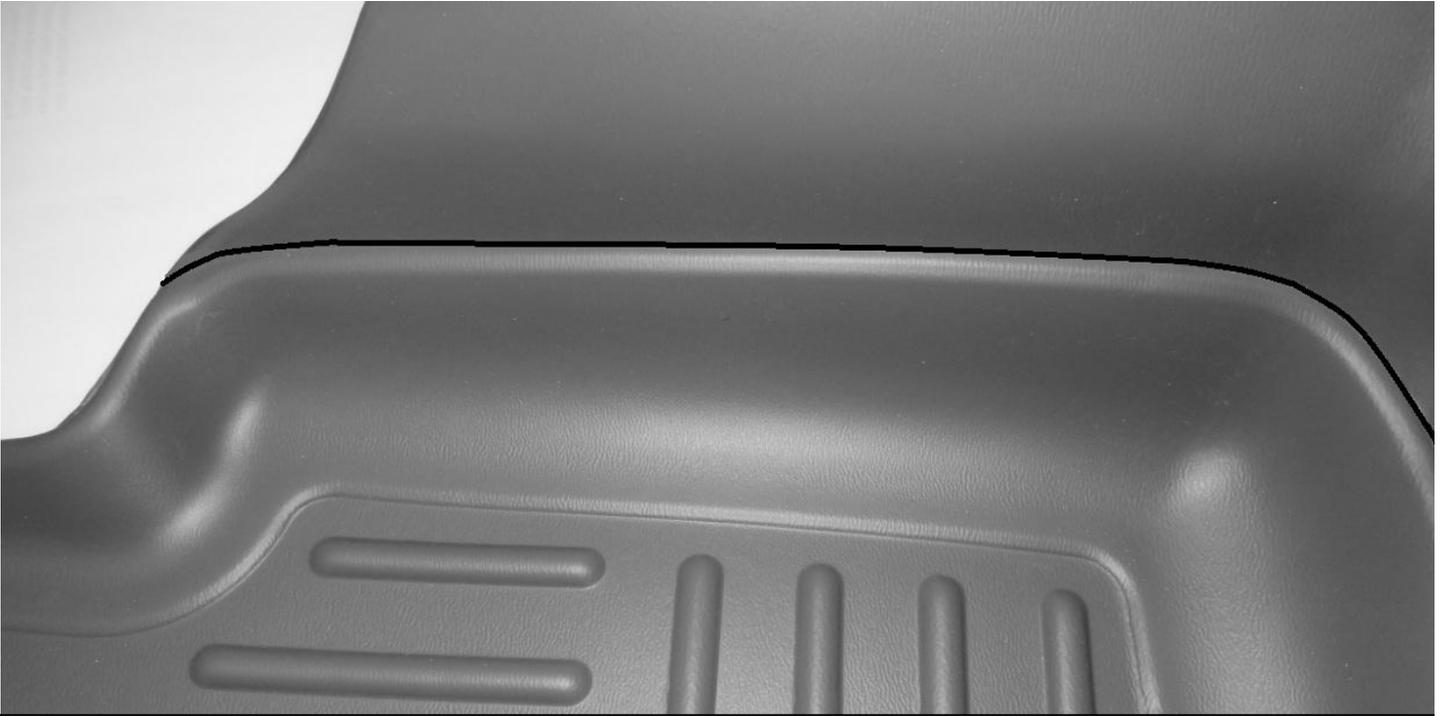
THE SOLID BLACK LINE ABOVE IS THE INTERSECTION FORMED BETWEEN THE CENTER HUMP AND THE FLOOR PAN SECTION OF THE LINER. USE THIS EDGE AS YOUR TRIMMING GUIDE. SCISSORS WORK WELL FOR TRIMMING. YOU WILL LEAVE THE EDGE ATTACHED TO THE FLOOR PAN PORTION OF THE PART—NOT THE CENTER HUMP COVER. BELOW IS A PHOTO OF THE TRIMMED FLOOR PAN SECTION. MAKE THIS TRIM ON BOTH SIDES OF THE LINER.
