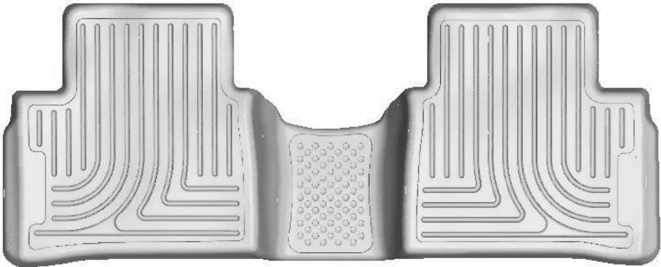
TO EASE INSTALLATION OF YOUR ALTIMA SECOND SEAT LINER, MOVE THE FRONT SEATS TO THEIR MOST FORWARD POSITIONS. WITH THIS DONE, INSERT LINER IN YOUR VEHICLE AS SHOWN IN THE IMAGE ABOVE. ONCE THE LINER IS INSTALLED, REPOSITION THE FRONT SEATS AS DESIRED.
