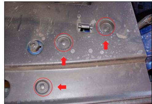
Remove the 3 push pins on the passenger side from the radiator shroud.
