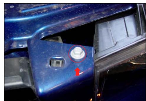
Remove the 10 mm screw from the top of the bumper located next to the headlight. Remove bumper by pulling straight out.
