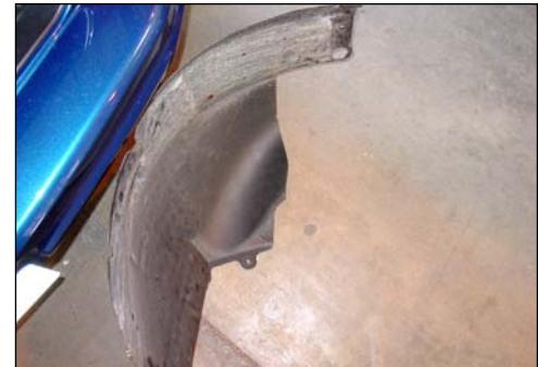
Remove the fender from the vehicle.
