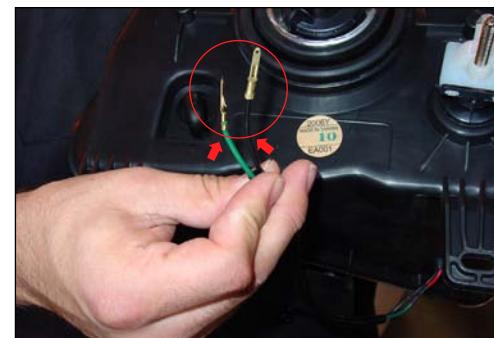
On the Anzo USA™ headlight assembly the HALO will have exposed plugs, cut the plugs off.
