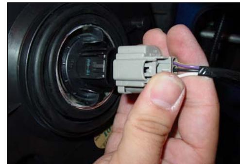
Pull the headlight housing straight out and disconnect the harness from the headlight bulb.
