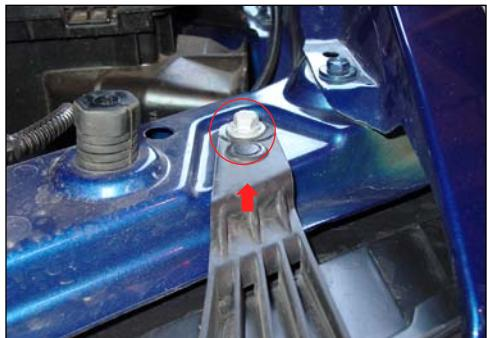
Remove the 10 mm screw located on the top of the headlight.
